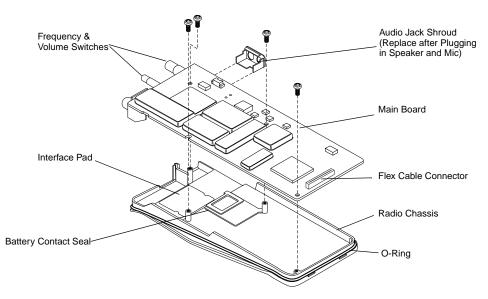
Figure 6-17. Main Board onto Chassis Re-assembly
