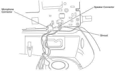
Figure 7-18. Microphone and Speaker Wires
