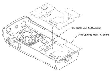
Figure 6-15. LCD/Keypad Board Re-assembly
