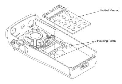
Figure 7-14. Keypad Re-assembly
