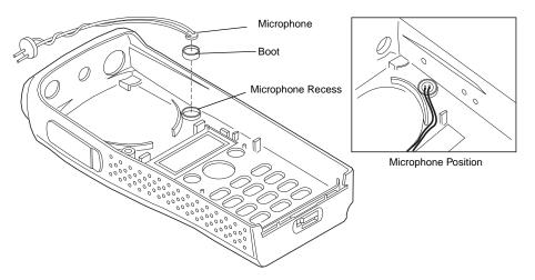
Figure 6-12. Microphone Re-assembly
