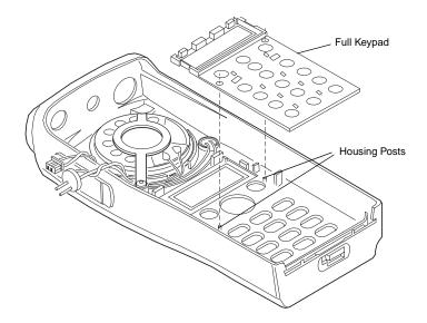
Figure 6-14. Keypad Re-assembly
