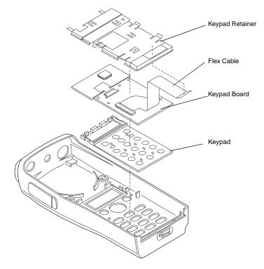
Figure 6-8. Keypad Removal
