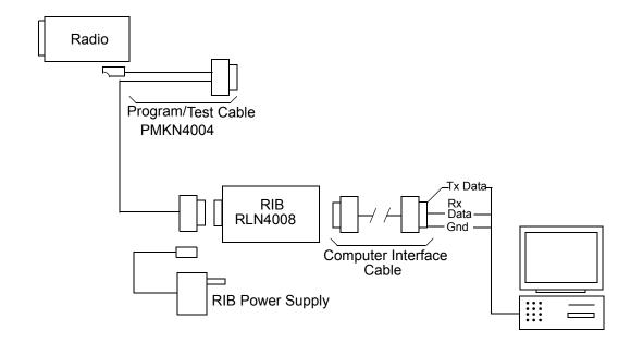
Figure 4-1. Radio Performance Checks Setup
