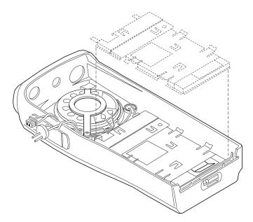
Figure 6-16. Keyboard Retainer Re-assembly
