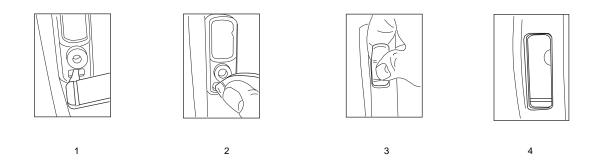
Figure 8-9. Dust Cap Re-assembly
