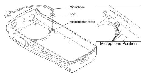
Figure 8-10. Microphone Re-assembly
