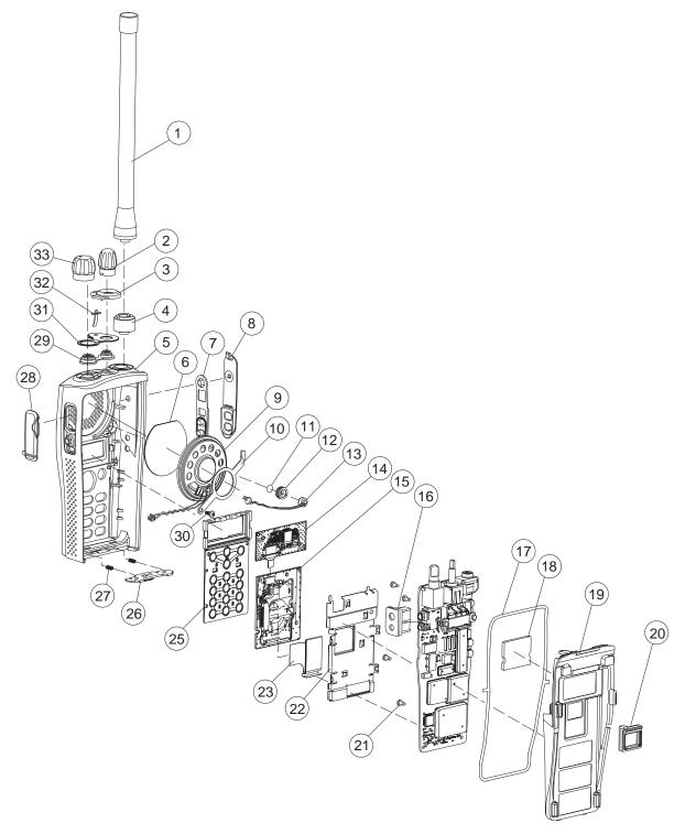
Figure 6-22. PR400 Full Keypad Radio Exploded View
