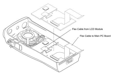
Figure 7-15. LCD/Keypad Board Re-assembly
