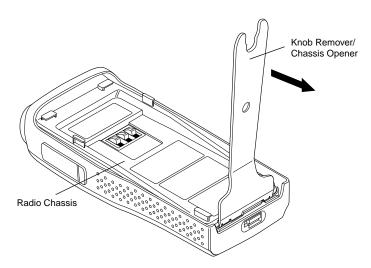
Figure 8-3. Chassis Removal
