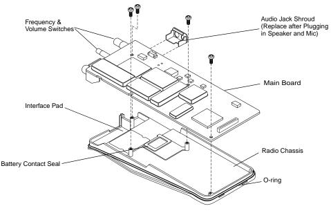
Figure 8-12. Installation of Main Board onto Chassis
