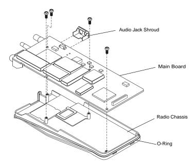
Figure 8-8. Removal of Main Board from Chassis
