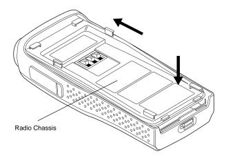
Figure 7-20. Fastening the Chassis
