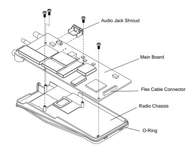
Figure 7-10. Removal of Main Board from Chassis
