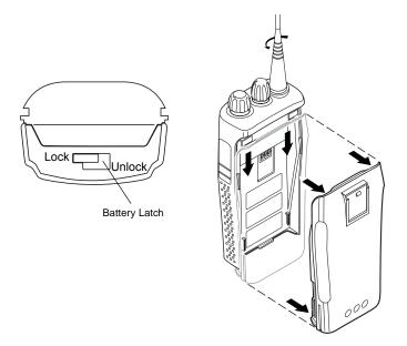
Figure 8-1. Battery Removal
