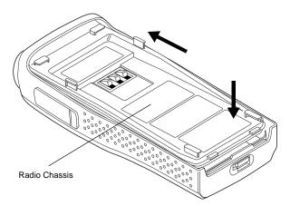
Figure 6-20. Fastening the Chassis
