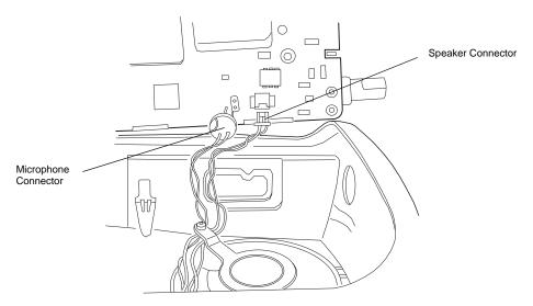
Figure 6-5. Microphone and Speaker Connections
