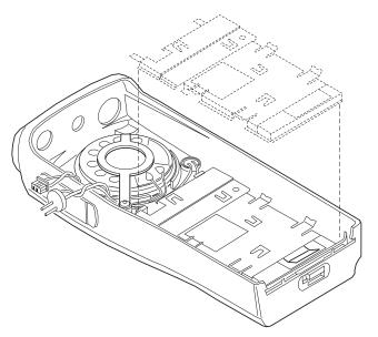
Figure 7-16. Keyboard Retainer Re-assembly
