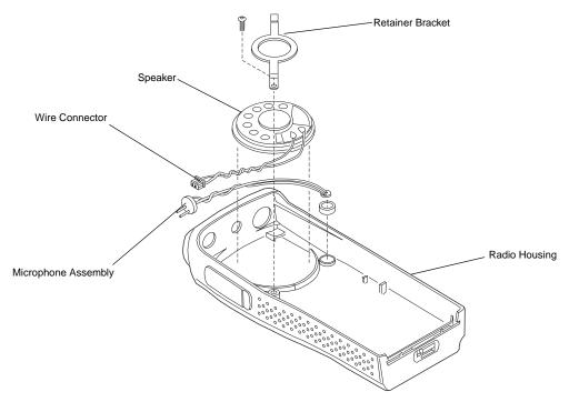
Figure 8-6. Removal Speaker-Microphone Assembly
