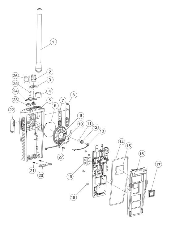
Figure 8-16. PR400 Non-Keypad Radio Exploded View
