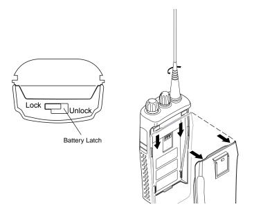
Figure 7-1. Battery Removal
