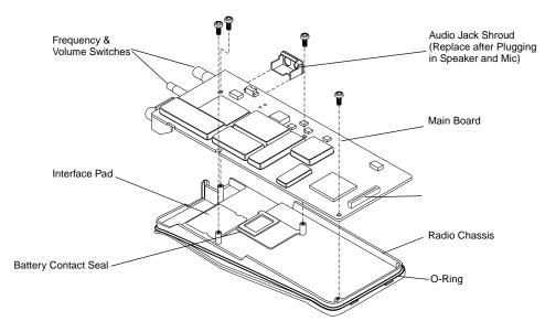
Figure 7-17. Installation of Main Board onto Chassis
