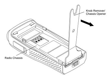
Figure 6-3. Chassis Removal
