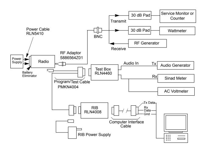
Figure 5-2. Radio Tuning Setup
