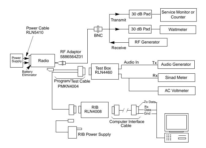
Figure 5-2. Radio Tuning Setup
