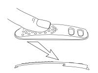
**b**. Push down on PTT toward bottom of radio so hooks do not get crushed.
