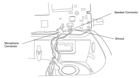
Figure 8-4. Microphone and Speaker Connections
