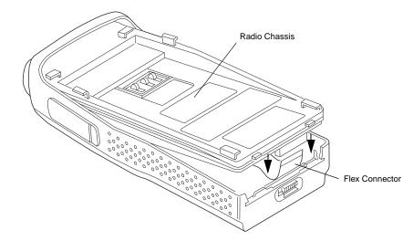
Figure 6-4. Keyboard Flex Connection
