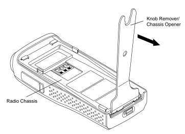
Figure 7-3. Chassis Removal
