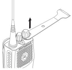
Figure 8-2. Antenna and Knob Removal
