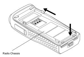
Figure 8-14. Fastening the Chassis
