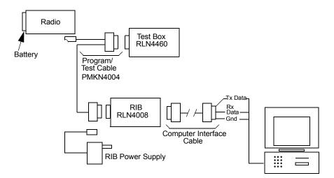
Figure 5-1. CPS Programming Setup
