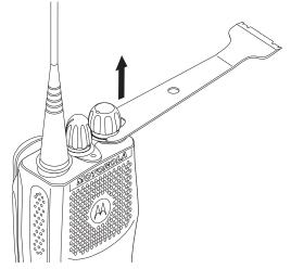
Figure 7-2. Antenna and Knob Removal
