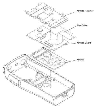
Figure 7-8. Keypad Removal
