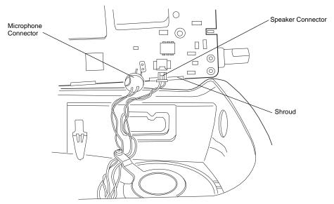
Figure 6-18. Microphone and Speaker Wires Re-assembly
