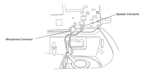
Figure 7-5. Microphone and Speaker Connections
