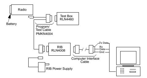
Figure 5-1. CPS Programming Setup
