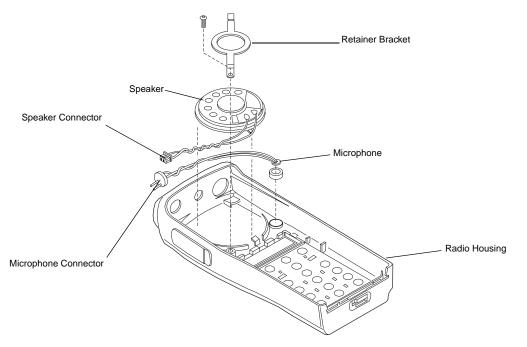
Figure 6-7. Removal Speaker-Microphone Assembly
