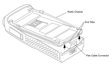
Figure 7-19. Keyboard Flex Cable Connection
