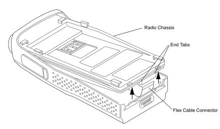
Figure 6-19. Keyboard Flex Cable Connection
