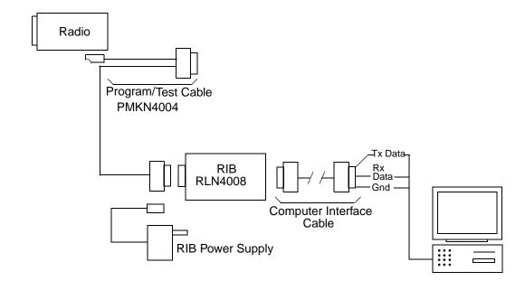
Figure 4-1. Radio Performance Checks Setup
