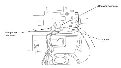
Figure 8-13. Microphone and Speaker Wires Re-assembly
