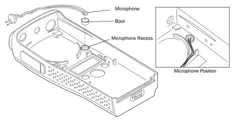
Figure 7-12. Microphone Re-assembly
