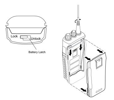
Figure 6-1. Battery Removal
