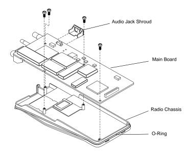
Figure 6-10. Removal of Main Board from Chassis
