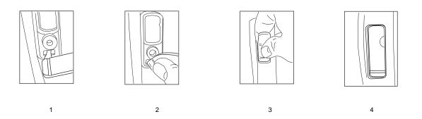
Figure 7-11. Dust Cap Re-assembly
