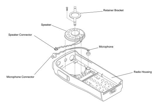
Figure 7-7. Removal Speaker-Microphone Assembly
