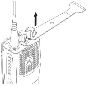
Figure 6-2. Antenna and Knob Removal
