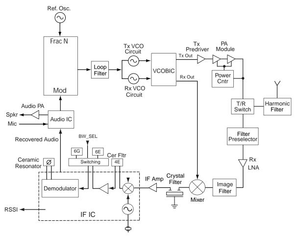
Figure 2-2. Transceiver Block Diagram
