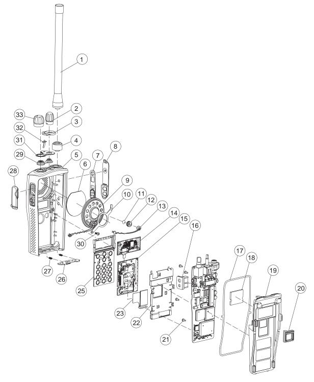
Figure 7-22. PR400 Limited Keypad Radio Exploded View
