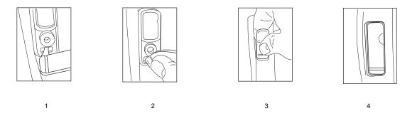
Figure 6-11. Dust Cap Re-assembly
