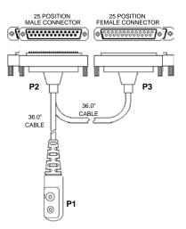
Figure 3-1. Programming/Test Cable
